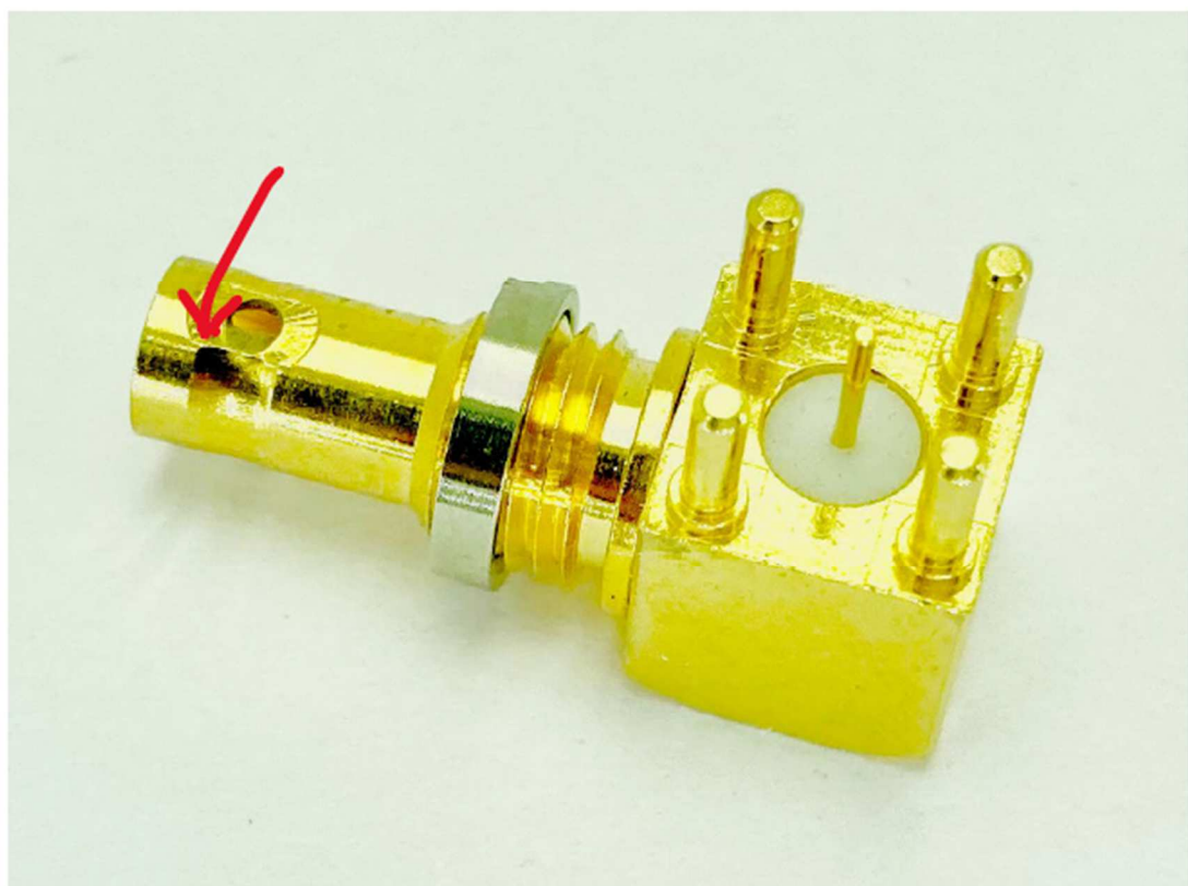
Image 4 – Photograph demonstrating where on connector breakage occurs with more than 1.0 Newton Metres of sheer force applied.
